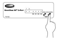
Pressing the CHANNEL button cycles you through all the ports, including inactive ports.
